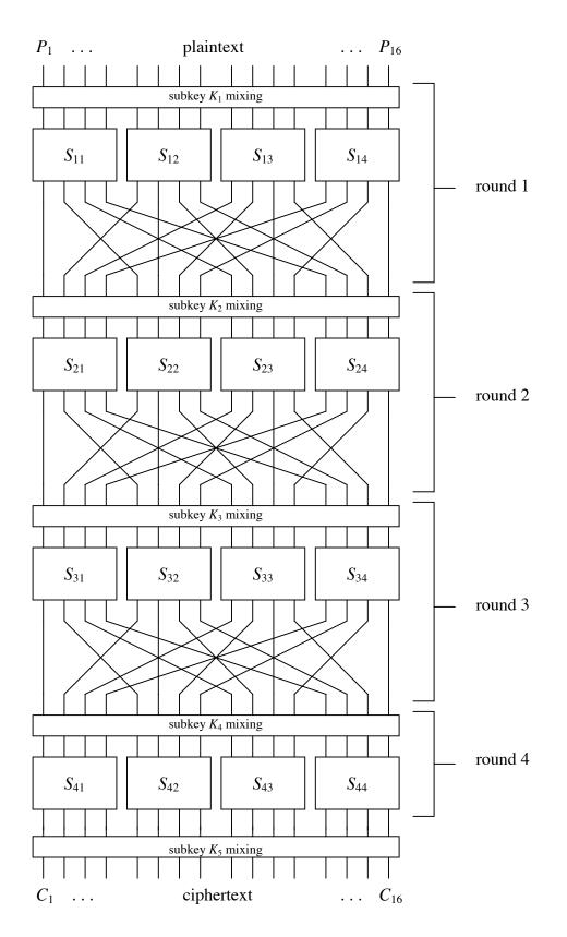
Figure 1. Basic Substitution-Permutation Network (SPN) Cipher
