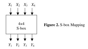
For example, for the S-box used in our cipher, consider the linear expression  $X_2 \oplus X_3 \oplus Y_1 \oplus Y_3 \oplus Y_4 = 0$  or equivalently
